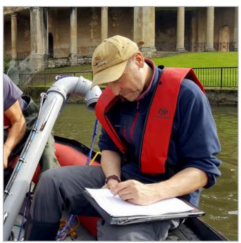
Stonbury completed two invertebrate surveys on the River Avon to sample above and below discharge points, using a Yorkshire Pattern' airlift pump.
